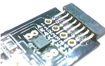
Solder the female header strip to the pads on the circuit board.
