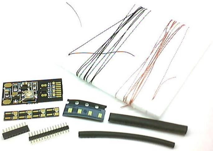
The DIY Kit Version allows people with the ability to do micro soldering, to build their own units. Note that this kit can't be soldered with a regular soldering iron due to the 1mm pitch connectors and pads on the circuit board, you will need a micro soldering iron.
