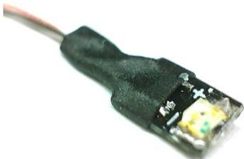
Cut a 5mm long piece from the 3mm heat shrink and squeeze it to slide it over the board where the wires are soldered on. You may need to file the rear corners of the board to allow the heat shrink to slide onto the board. Heat and press the sides together.
