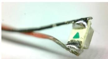
You may optionally prefer to solder the wires directly to the LED terminals to reduce weight or assist with fitting the LEDs.
