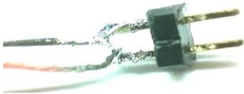
Solder the wires to the connector
