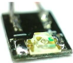
Solder the LED to the LED mounting board
