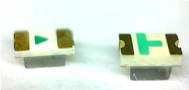
Turn the LEDs over to see the correct polarity. Align the arrow on the back of the LED to face the same direction as the one on the LED mount board. Both the LEDs in the image to the left have their polarity the same way.
