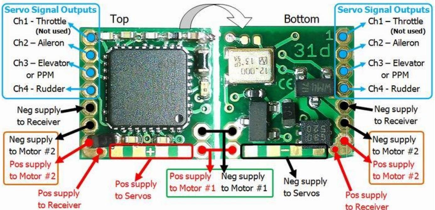
Channel 1 Throttle is not needed as this is handled by the onboard speed controllers. When differential steering mode is set with the transmitter, yaw is controlled by varying the power to each engine. You can choose whether the rudder or aileron will control the yaw. Normally, with this setup you would just have 2 motors and an elevator servo to control the plane.
