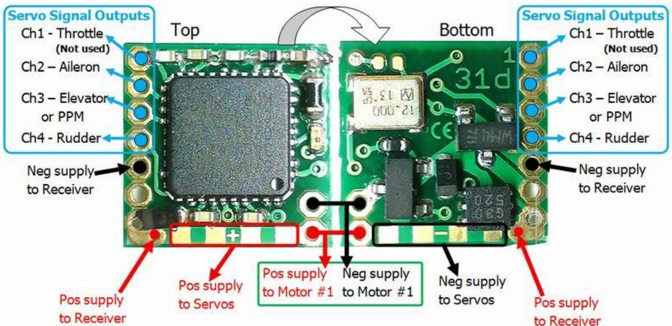
This is the most simple and straight forward system to set up. Note that the Ch1 - Throttle signal output is not needed as the onboard speed controllers take care of this. Also, in the image above we have connected the motor to one of the speed controller connectors. However, it doesn't matter which one you connect the motor to.
