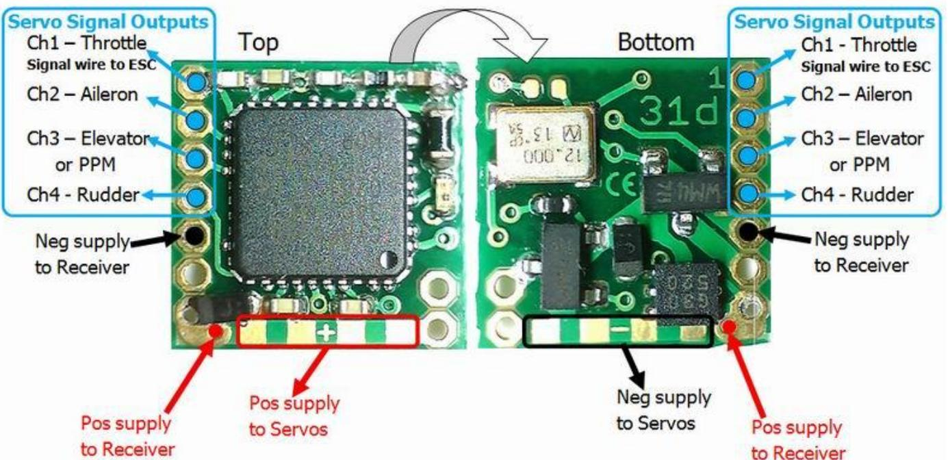
The configuration above is an example of a simple set up for a plane with aileron, rudder and elevator controls as well as a single brushless motor. In this setup, a signal wire from Ch1 – Throttle goes to the signal port on your ESC unit. Note that power to the ESC unit may be supplied with leads from the receiver but in the example above we have assumed that the pos and neg power to the ESC unit will be supplied with leads direct from the battery.
