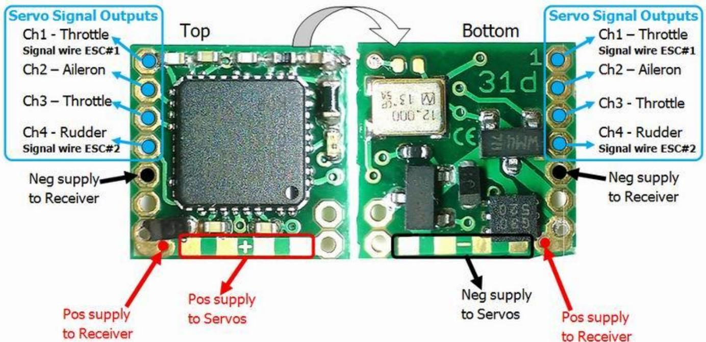
This example shows a common setup for running a system with dual brushless motors. Note that you will also need 2 ESC units. Once the receiver has been set for differential steering by using the transmitter, the signal for the ESC units will be provided from Ch1 and Ch4 on the receiver. You can choose whether the rudder or ailerons control the differential steering. With this setup you would typically have 2 motors and their ESC units and one servo for the elevator.
