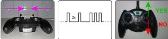
1. Switch Transmitter on with left/right sticks in towards middle of Tx.
