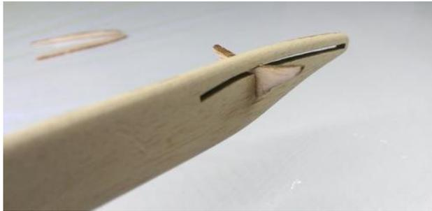
Glue in the wing support. Note that the wing support will completely block the wing slot in the main fuselage. This is how it is supposed to be. Refer to the slots in the wings to see how they attach.
