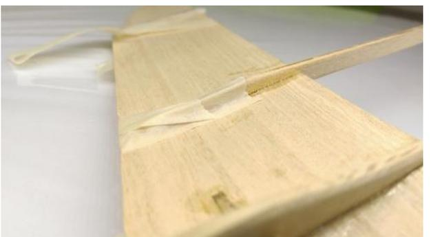
Once the previous step has completely dried, continue to glue the rest of the tail shafts to the leading part of the wing. You can use masking tape as shown here to hold the wing down onto the tail shaft. Or you can use clips as shown below.
