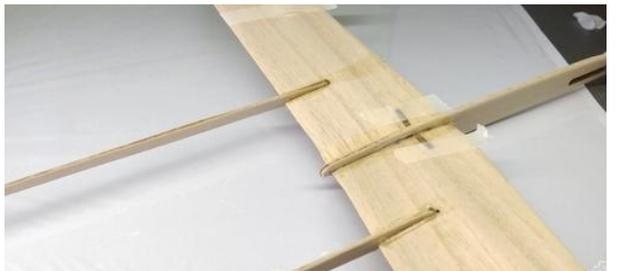
Glue in place the tail shafts. Only glue the part on top of the wing as well as the rear 1cm under the wing.
