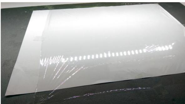
Firstly it's a good idea to tape down a sheet of cling wrap over your work surface. This will stop the parts from becoming glued to the surface. It's easier to peel off cling wrap from any wooden parts.
