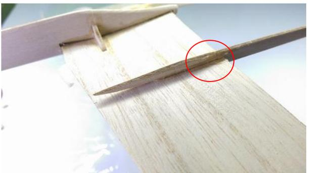
Only glue 1cm at the back of the wing underneath, and allow to dry.
