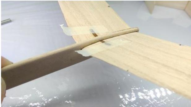
Glue the wings in place into the main fuselage ensuring they are both inserted an even amount. Ensure that you apply glue around the wing mount and put masking tape over the top like this to make sure the wings stay up while drying.
