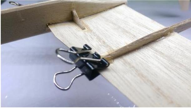
Alternate method of holding the wing to the tail shaft as it dries.
