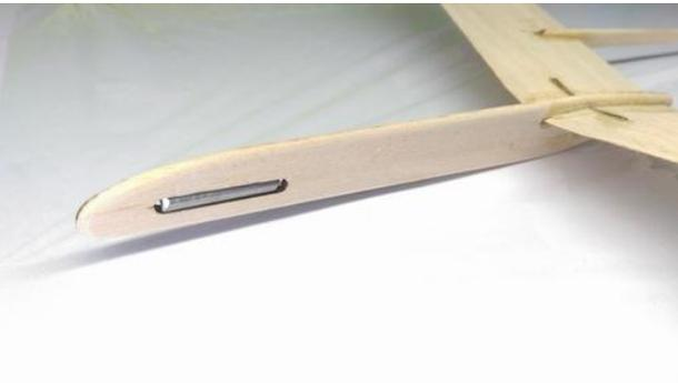
Place the ballast in the nose and hold it in place with tape while test flying.
