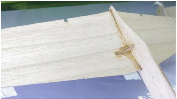
Also reinforce the joint with some extra glue under the wings.
