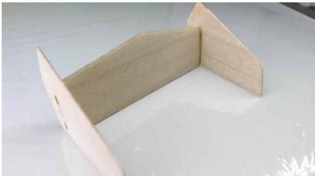
Glue on the vertical stabilisers to the horizontal stabiliser and make sure they are perpendicular (90 degree angles). Then place them down like this to dry.
