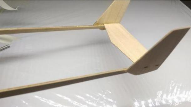
Glue in place the tail section as shown here on top of the tail shafts.
