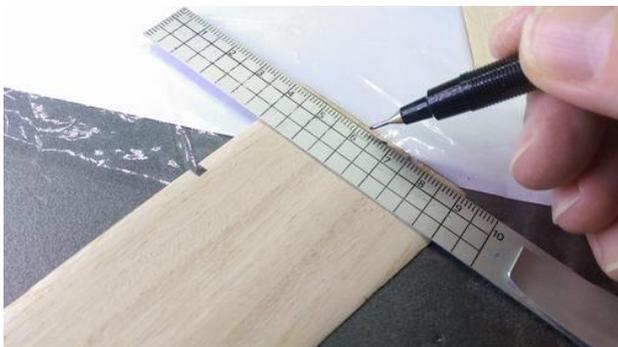
Each wing must be inserted half way into the body part, so mark a line about 2mm from the end of the wing. This will help when inserting the wings to make sure you have each wing inserted the same amount.
